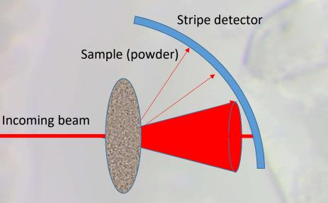
In reality: intensity from a powder is emitted in a cone; the stripe detector is cutting out a small part of it
