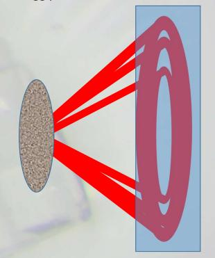
A flat 2D detector ("Camera") cold detect the complete beamcone, increasing by a factor of 100-1000 the detected flux, eventually sacrificing range in reciprocal space
